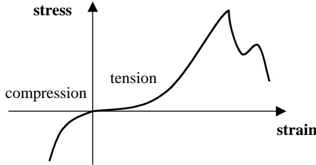
Figure 5 : typical stress-strain-diagram for biological media
